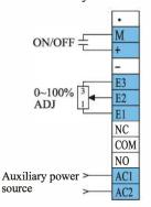
5. Manual-automatic relay switch, outside VR adjustment
