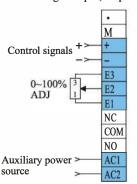
4. Dry contact signal input, outside VR adjustment
