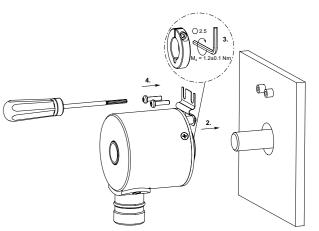
All movable adjusting elements need tolerance in both axial and radial direction in order to equalize shifts by temperature and of mechanical nature. Tighten both fixing and clamping ring screws firmly. The torque support is not allowed to have any contact to the encoder or motor except on the mounting point.
